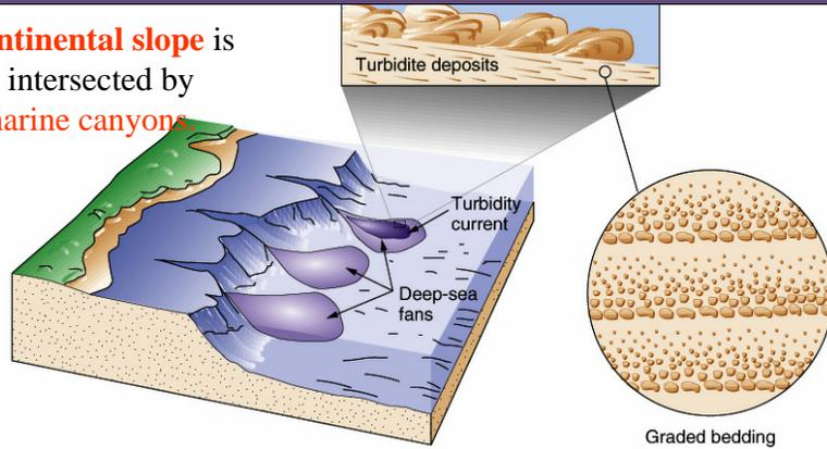
Fig. 4-9. Turbidity currents move downslope and erode submarine canyons in the continental slope.
